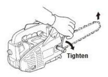
While lifting the chain guide, turn the content screw to apply correct tension to the chain.
