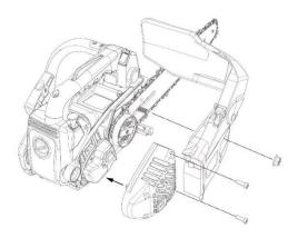
7) Adjust the chain tension by turning the tension screw until the straps touch just the bottom side of the bar.
