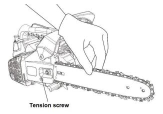
8) Tighten the nuts and check if the chain is rotated correctly and tight.
