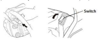
c. Pull the starter button. The starter will close and the throttle will be moved to the starting position
